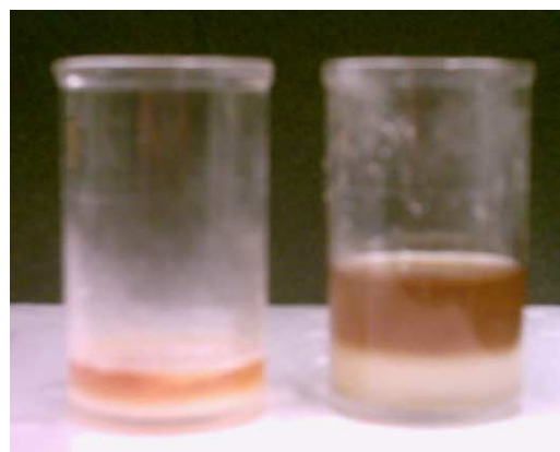
Fig. 9. Anolyte (right) and catholyte (left) of the EKD of gravity pre-thickened sludge.
